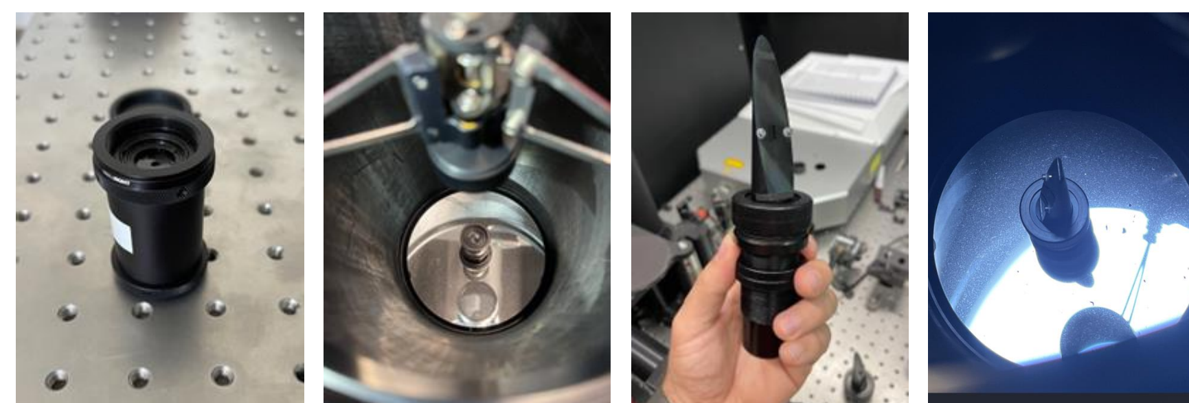
Figure 2: Normal field stop vs tilted slit. Upper-left: normal circular field stop; Up-right: field stop inside the telescope; Lower-left: tilted slit solution; Lower-right: tilted slit installed inside the telescope.
